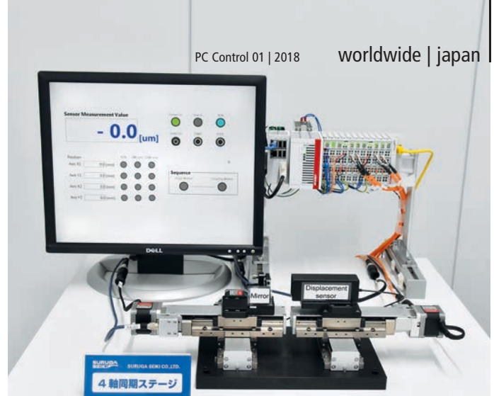
Example application of a precision positioner: the CX5140 Embedded PC helps achieve a synchronization accuracy of \pm 1.0 \mu\text{m} with four-axis synchronization control.
