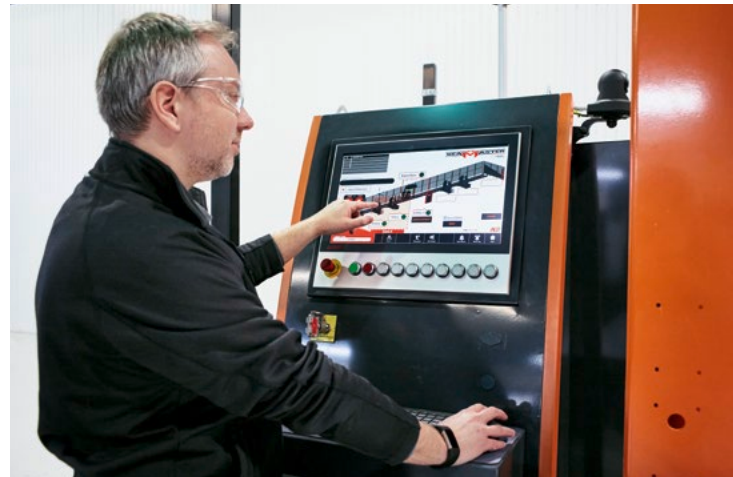
AGT Robotics implemented a CP2918 multi-touch Control Panel from Beckhoff for the system's operator interface.
