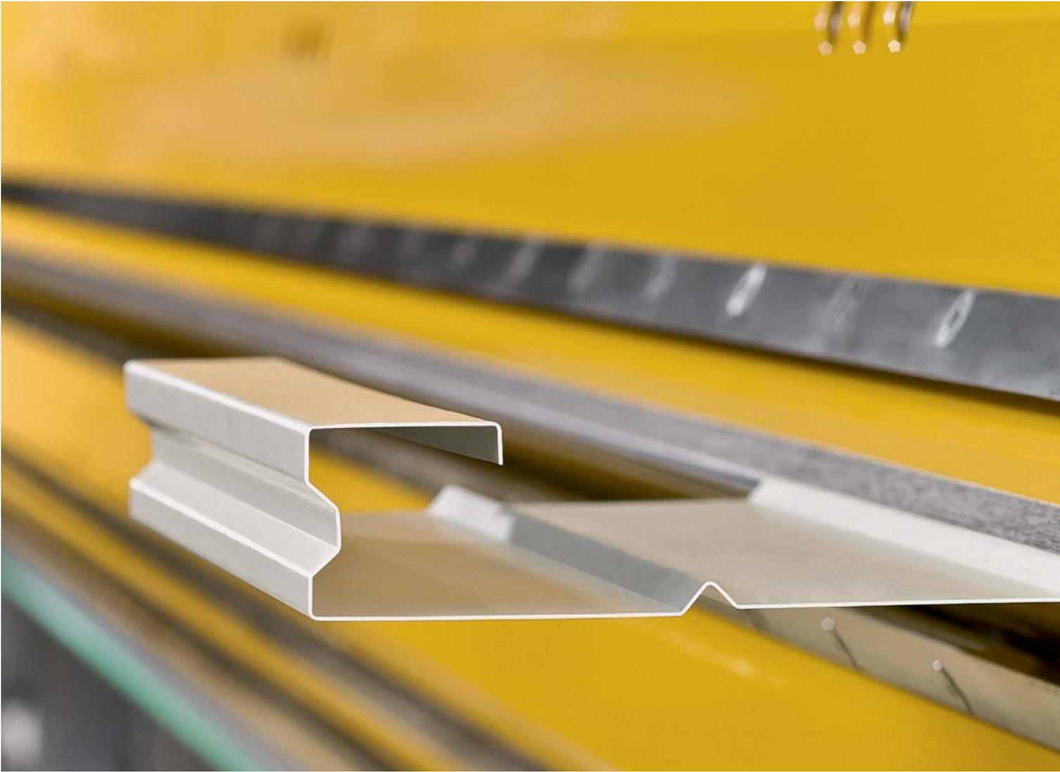
Embedded PC controls double bending machine
