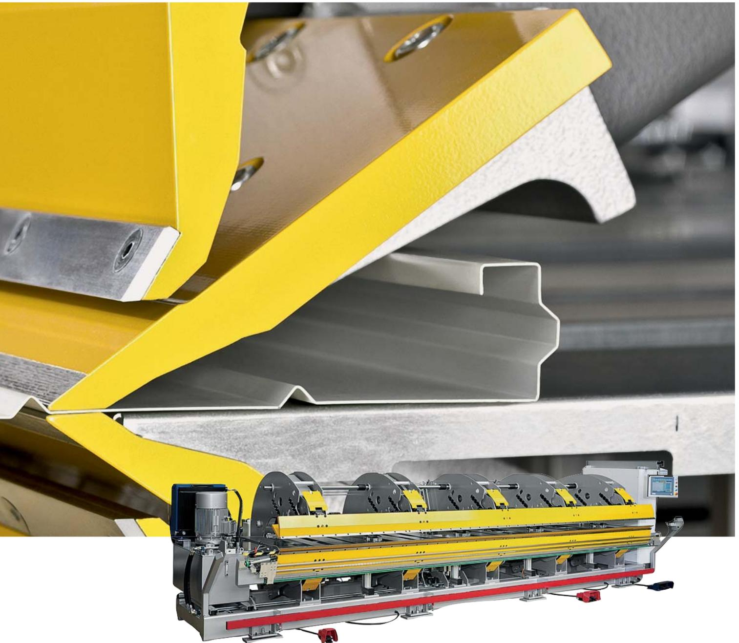
**TD-150 double bender:** Thalmann's control-shaft technology ensures highly accurate bending results. The double bender achieves accuracies of up to  $\pm 0.5^\circ$  ( $\pm 1^\circ$  with basic models) at a maximum bending angle of up to  $143^\circ$  and, thanks to high-performance hydraulics, amazingly needs just three seconds for the combined outward- and return stroke.
