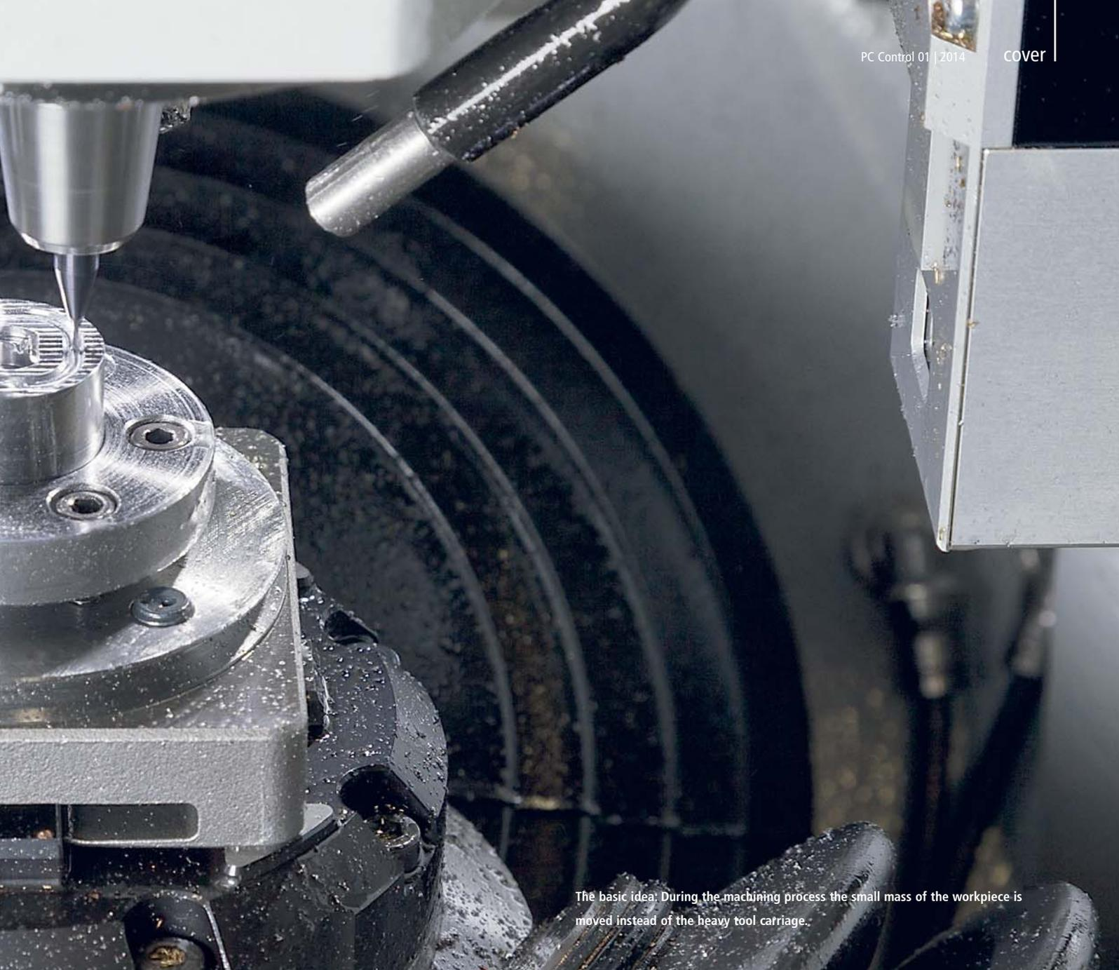
The basic idea: During the machining process the small mass of the workpiece is moved instead of the heavy tool carriage.
