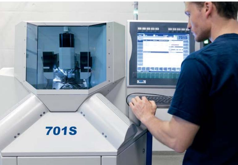
The machining center is operated via a customized CP7912 "Economy" Control Panel with 15-inch touch screen.
