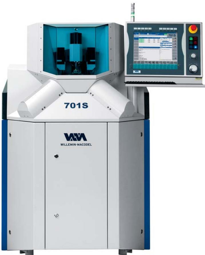
tationally intensive "circular interpolation". The key characteristics include path accuracy better than 0.2  $\mu\text{m}$ , low sensitivity to temperature fluctuations as well as very high precision and repeatability. A specially designed high-performance motor spindle, with a maximum speed of 80,000 rpm and without tool holders, additionally provides increased static and dynamic rigidity, very high balancing quality and a low radial runout (less than 1  $\mu\text{m}$  at the tool tip).
