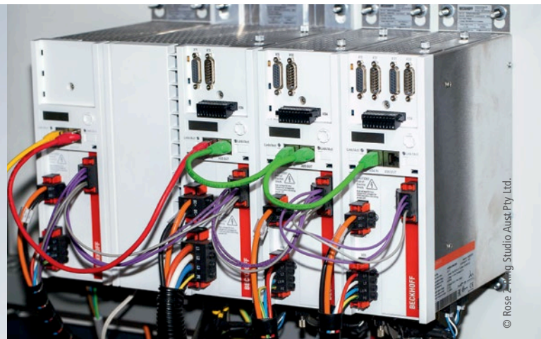
The AX5000 Servo Drives precisely control the AM8000 servomotors.
