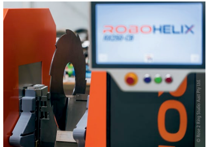
RoboHelix machines can form helical flights from standard circular or patterned blanks.
