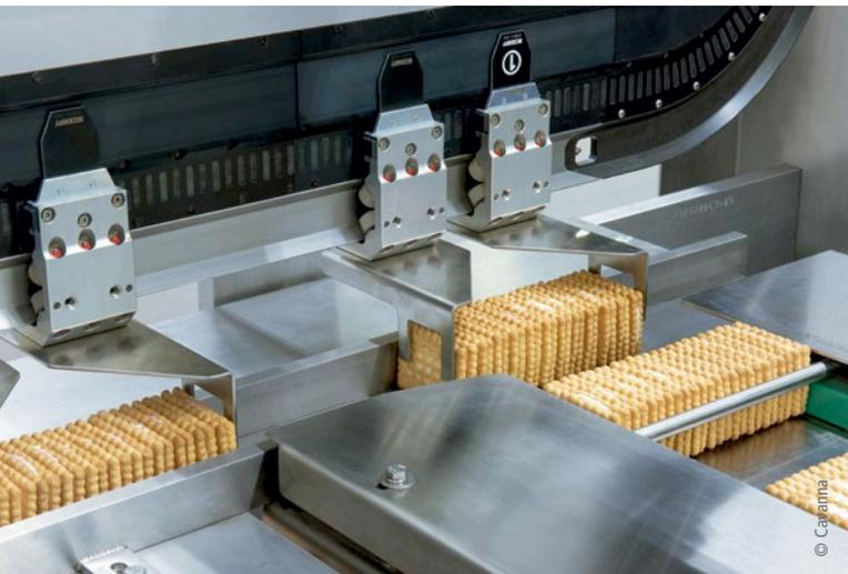
The slugs get tilted by 90 degrees before being handled by the XTS movers.
