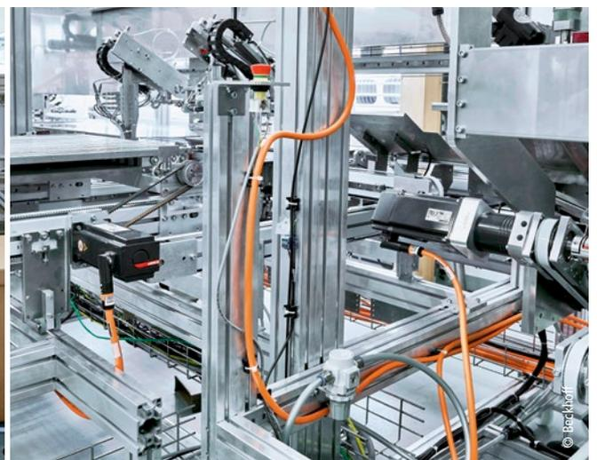
More than 100 drive axes implemented with AM8000 servomotors enable the numerous movements necessary to produce the packaging, transport the goods and insert the articles into the packaging.
