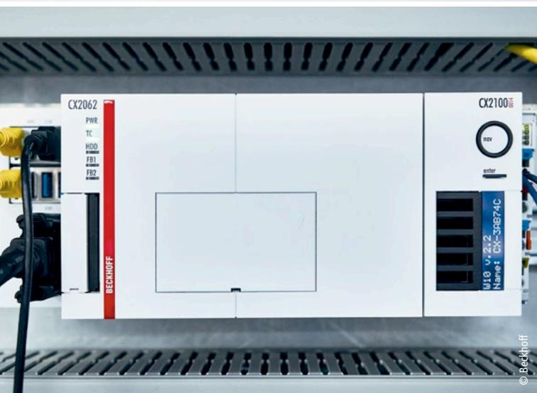
The system is controlled by a CX2062 Embedded PC.
