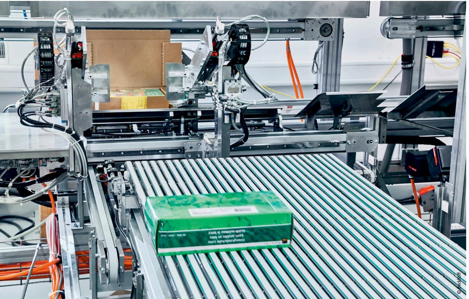
The PackOnTime® system merges the articles fully automatically with the tailor-made packaging.
