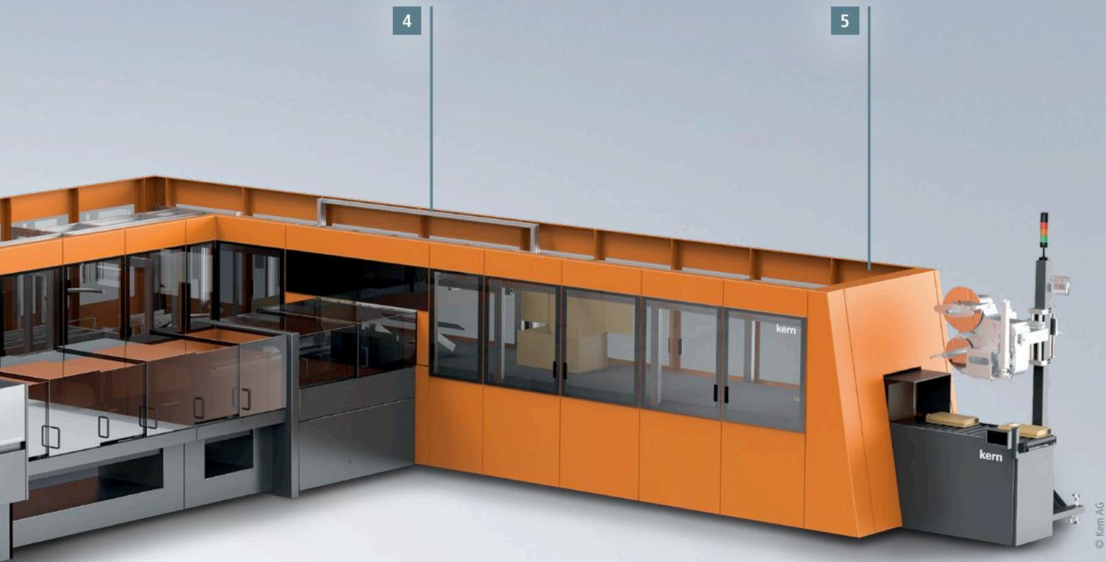
The PackOnTime® system consists of various modules: Placing and measuring (1), feeding the corrugated board (2), processing the corrugated board (3), packing the articles (4) and closing the packaging (5).
