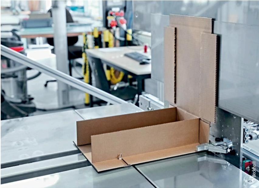
The corrugated cardboard is cut to size, perforated and grooved to perfectly match the contents; the packaging can then be assembled, glued and transported to the insertion station.
