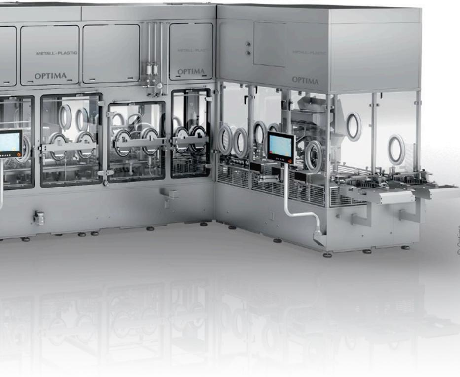
Optima offers optional smart features that can be added easily to its extensive range of pharmaceutical production systems using ultra-compact Industrial PCs from Beckhoff.
