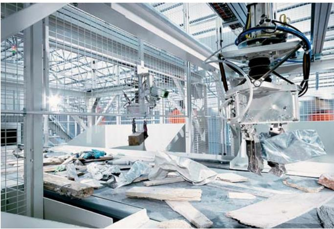
The recycling system from ZenRobotics uses self-learning robots to separate recyclable materials from the waste stream with high speed and efficiency.
