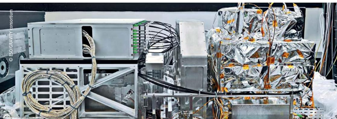
Gravity is a second-generation instrument for the VLT Interferometer and will enable measurement of the positions and movements of astronomical objects on much smaller scales than currently possible.
