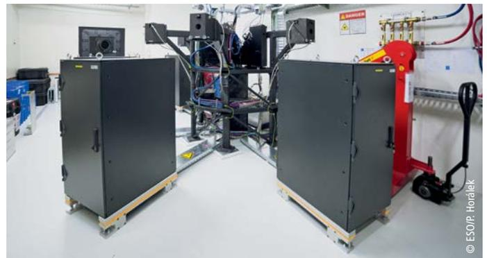
The Echelle Spectrograph for Rocky Exoplanet and Stable Spectroscopic Observations (Espresso) installed at the VLT allows the search for exoplanets to be carried out with unprecedented precision.
