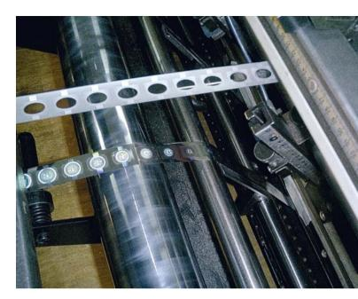
The position of the laser marking on the aluminum foil is logged quickly and exactly. It is then forwarded to the controller via the EtherCAT incremental encoder terminal.
