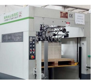
The fully automatic hologram foil stamping system integrates seamlessly into the punching and folding machine.
