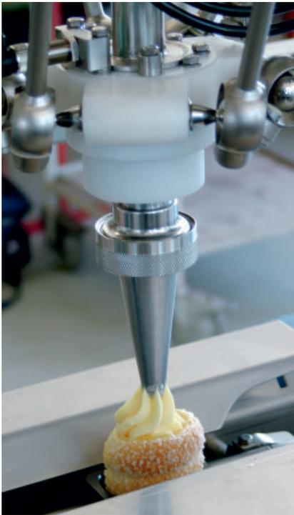
The pastry cases are fed into the filling machine upright, placed at a specific height and a specific distance apart.
