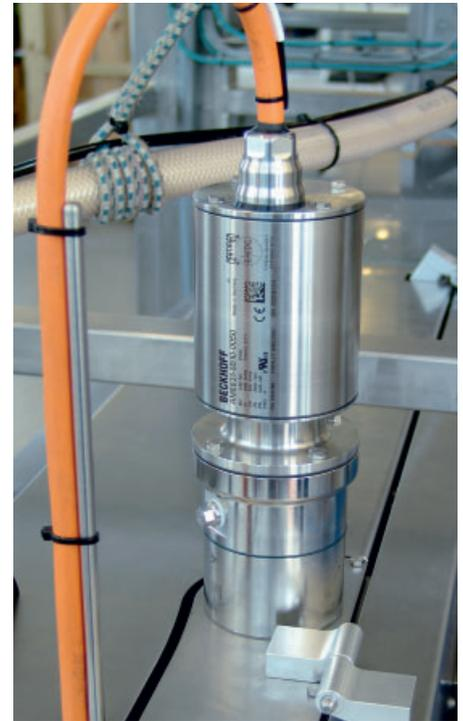
The control system of the filling station also integrates AM8831 servomotors with EHEDG-certified stainless steel housings
