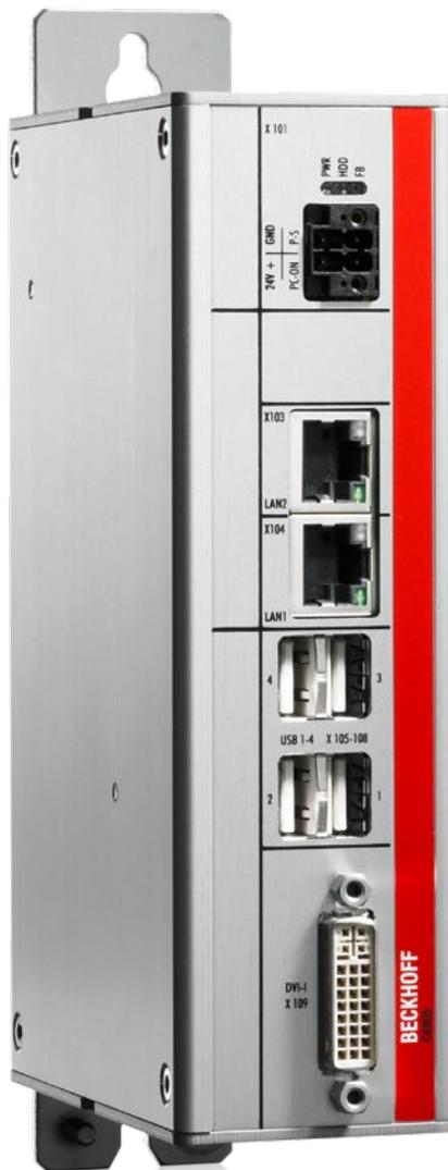
The Beckhoff CP6706 Panel PC and C6905 control cabinet PC tap into the computing power of the Intel® Atom™ multi-core processors for cost-sensitive applications.
