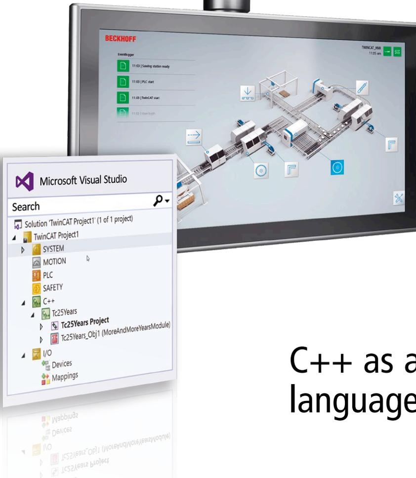
High-level language programming is seamlessly integrated into the development of the control project with TwinCAT C++.
