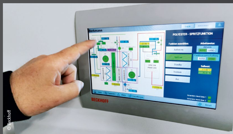
The Beckhoff CP690x built-in touch panel provides a clear, convenient location from which to visualize and operate the varnishing plant using the HTML5-based TwinCAT HMI.
